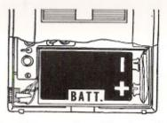
CAUTION: Install battery only in direction indicated or radio circuitry may be seriously damaged.
